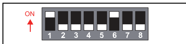
Figure 2-12 "Accept" Mode DIP Switch Settings
